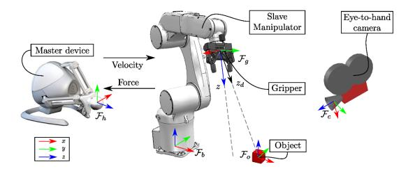
**Problem**: reduce the operator's workload during sort and segregation of nuclear waste
