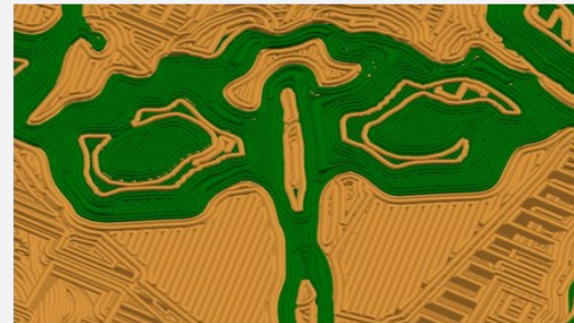
Layer 3 – Support structures
