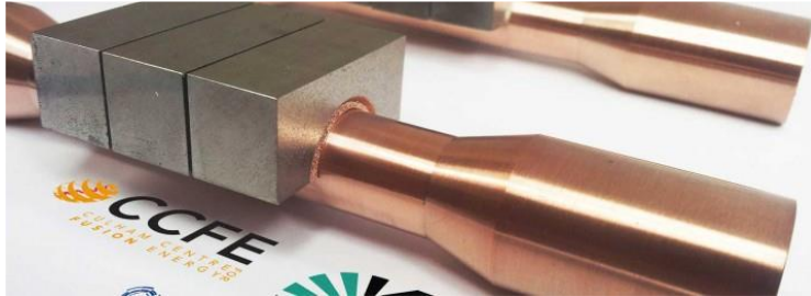
Water-cooled tungsten mock-ups produced by CCFE and KIT.
