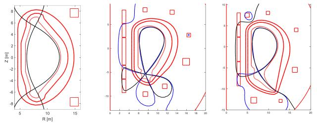
Once the optimized Alternative Magnetic Plasma Configurations have been designed, an assessment of the vertical stability properties have been carried out. In particular, for the different plasma configurations, open loop non-linear dynamic simulations have been produced taking into account the eddy currents originating in the passive structures and the presence of the ports (needed for the device maintenance).
