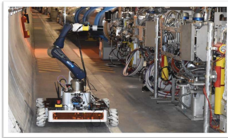
The CERNbot system during a test in front of a collimator of the LHC tunnel [5].
