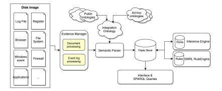
Our overall system consists of an ontology and five modules: Evidences Manager, Semantic Parser, Inference Engine, SWRL Rule Engine and a Query and Visualization module
